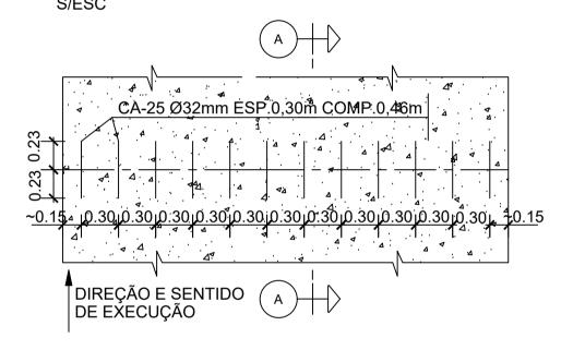
DETALHE "B" - TELA NERVURADA SOLDADA
